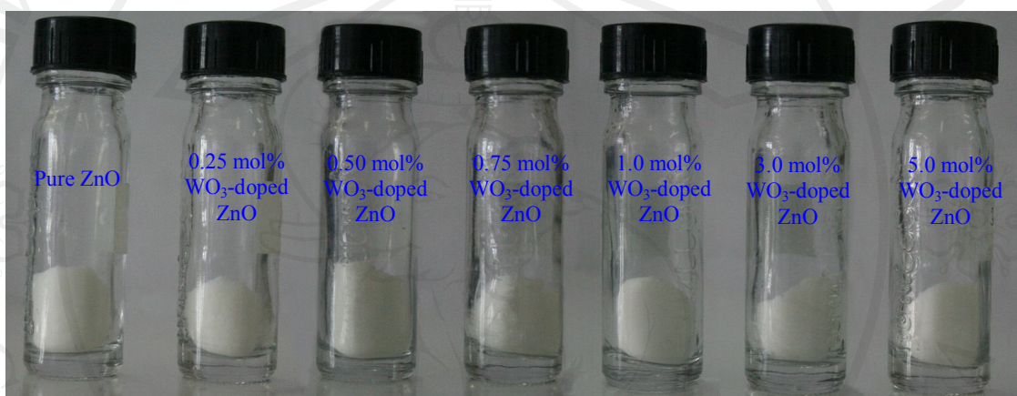
Figure 2.9 The flame-made (5/5) pure ZnO and 0.25-5 mol% WO 3 -doped ZnO nanoparticles ordered from the left to right with increasing WO 3 concentrations.
