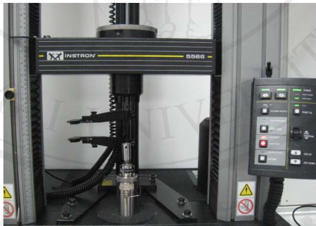
Figure 9 shows Universal Testing Machine (UTM) with the tensile bond testing apparatus.
