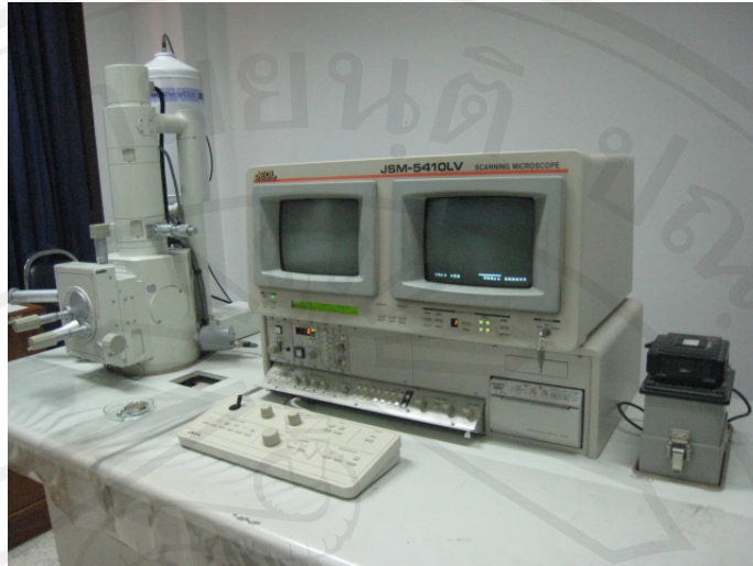
Figure 12 shows a Scanning Electron Microscope (JEOL® JSM-5410LV; JEOL, Tokyo, Japan).
