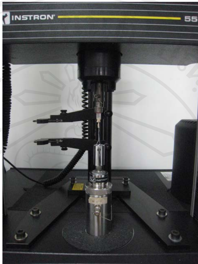
Figure 10 shows a specimen was fixed to the tensile bond testing apparatus.
