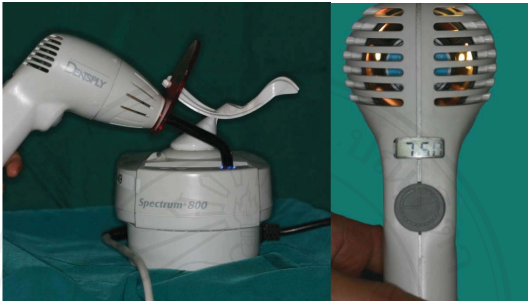
Figure 23 a. Checking light intensity for Spectrum 800 halogen curing unit, b. The screen showed intensity of the light
