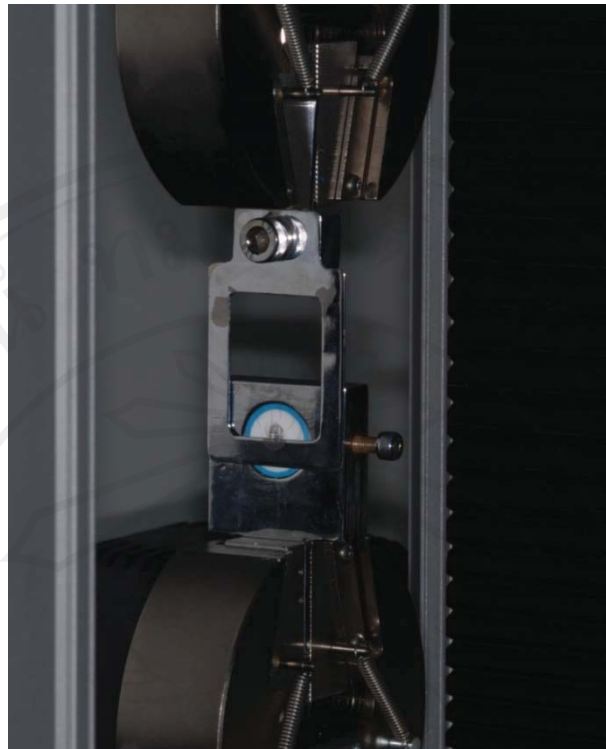
Figure 27 Polyvinylchloride ring mounted into mounting jig attached to the lower pneumatic grip with de-bonding plate attached to the upper pneumatic grip
