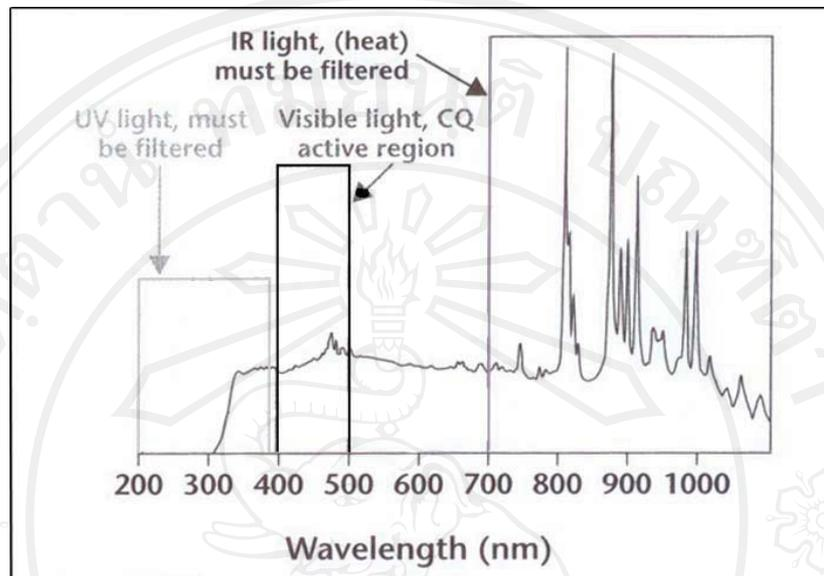
**Figure 2** Spectral emission of plasma arc light.
