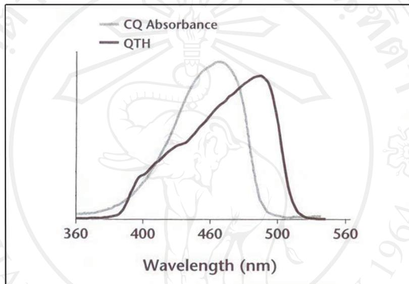
**Figure 1** Spectral emission of QTH lamp and camphorquinone absorbance.
