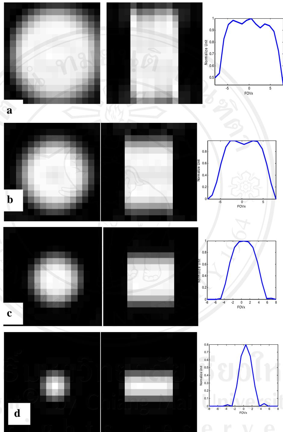
**Figure 4.7** Varying excitation FOV in x-y plane, this figure show images from the simulation in x-y (left), x-z planes (middle) and the 1D profile along FOVx (right). In x-y plane, full (4/4) excitation FOV the same as FOV of object (a), reduce excitation FOV to 3/4 (b), reduce excitation FOV to 2/4 (c) and reduce excitation FOV to 1/4 (d).
