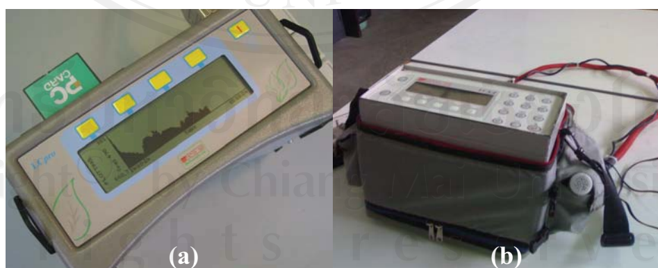
Figure 5.2 Measurement of photosynthetic efficiency using leaf chamber analyzer Model LCpro + , ADC BioScientific Ltd., Great Amwell, Herforshire England (a) and LCA4, ADC, Hoddessdon, Herts, England (b).
