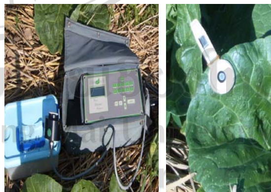
Figure 7.19 Fluorescent chlorophyll apparatus and sensor on cabbage leaf
