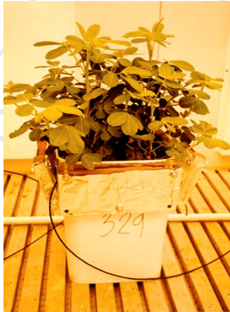
Figure 2.1 Photograph showing attachment of cuvettes to the sides of container.
